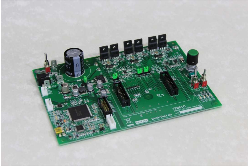
Fig 2 T2001C Low voltage inverter (Successor model of T2001B)
