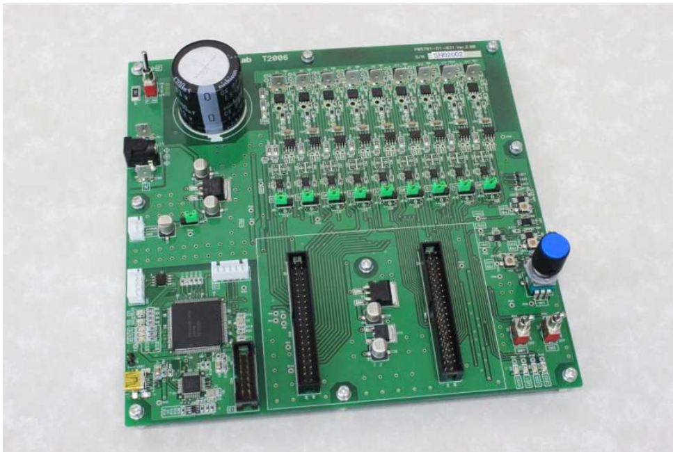
Fig 3 T2006A Low voltage inverter (Three phase inverter 3 port version)
